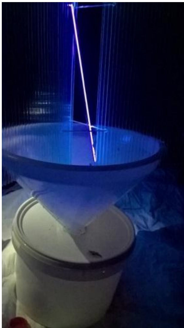
Figure 7. Alt – automatic light trap with UV cold cathode light switched on/off by timer (Photo: N.Tridrih)
