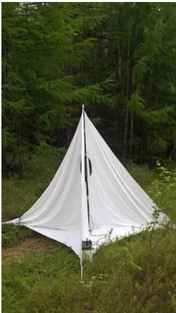
Figure 6. Mlt –pyramidal shaped white sheet screen with two 12V/8W UV (black light) fluorescent tubes (Photo: N.Tridrih)
